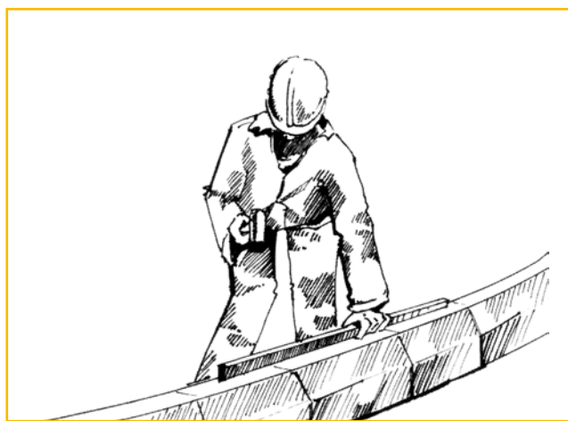
Figure 3: Checking of edge restraints
