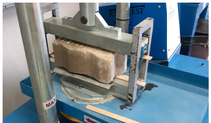
Tensile strength testing as applicable to SANS 1058:2021.
